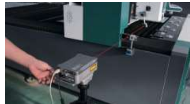
06 PRECISION INSPECTION Laser interferometer to ensure the overall machine precision.
